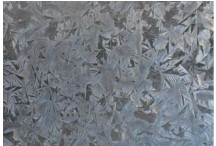
The distinctive "spangle" pattern of galvanised steel
